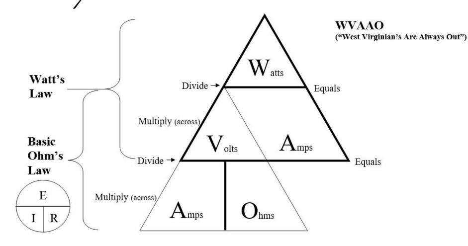
$W=Watts \ (P_{Power,\ Volt\ Amp}) \qquad \qquad A=Ampere \ (I_{Intensity,\ Current})$   $V=Volts \ (E_{Electromotive\ Force}) \qquad \qquad \Omega=Ohms \ (R_{Resistance})$
