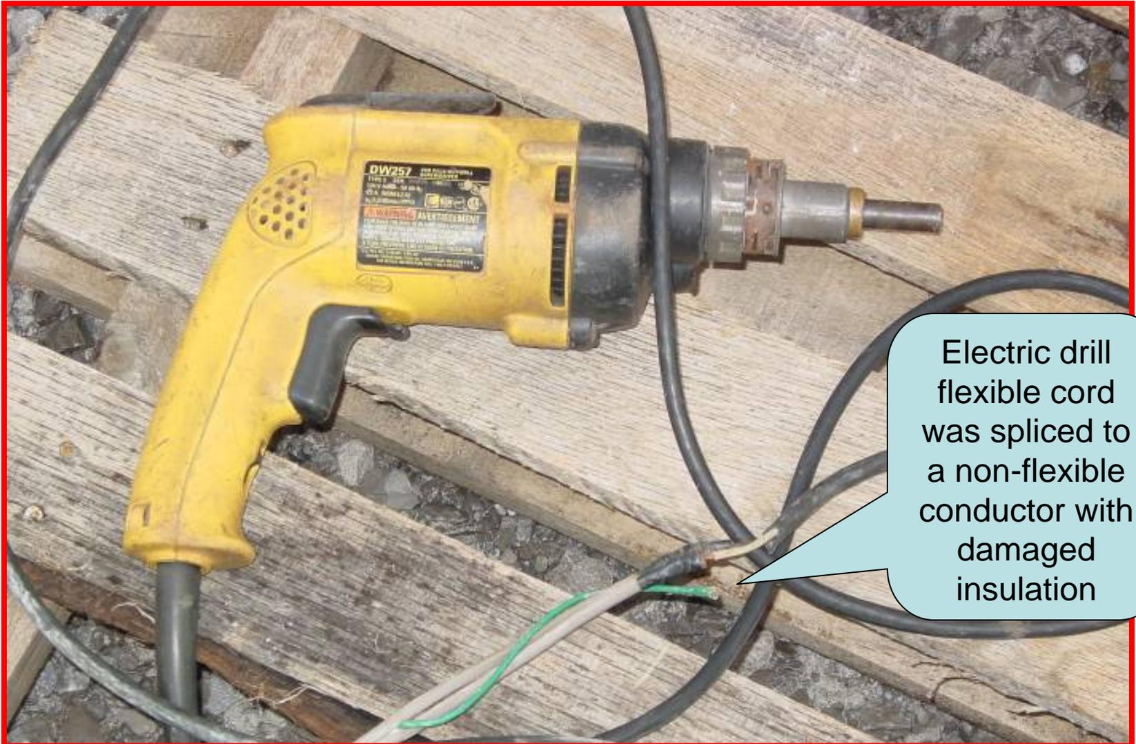
Electric drill flexible cord was spliced to a non-flexible conductor with damaged insulation
