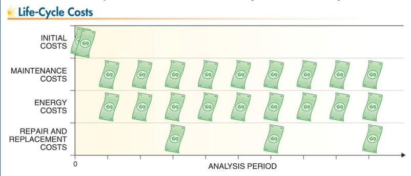
The life-cycle cost analysis of an enginegenerator system includes each type of cost.
