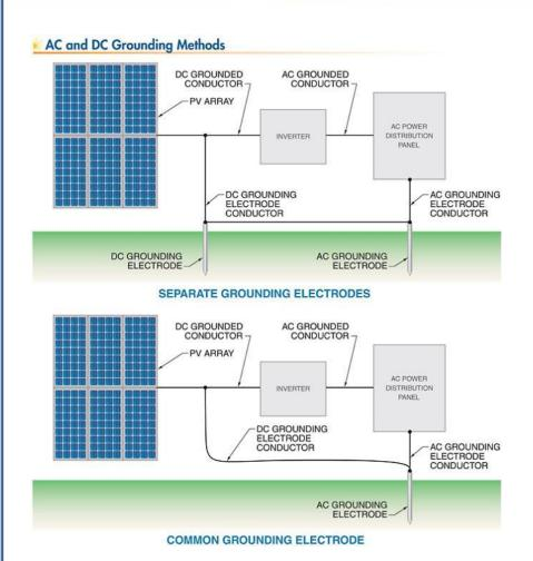
There are two acceptable methods of grounding both the AC and DC sides of a PV system.
