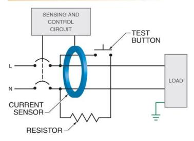
A ground-fault circuit interrupter (GFCI) senses differences between the current in the grounded and ungrounded conductors, indicating a ground fault, and opens the circuit in response.
