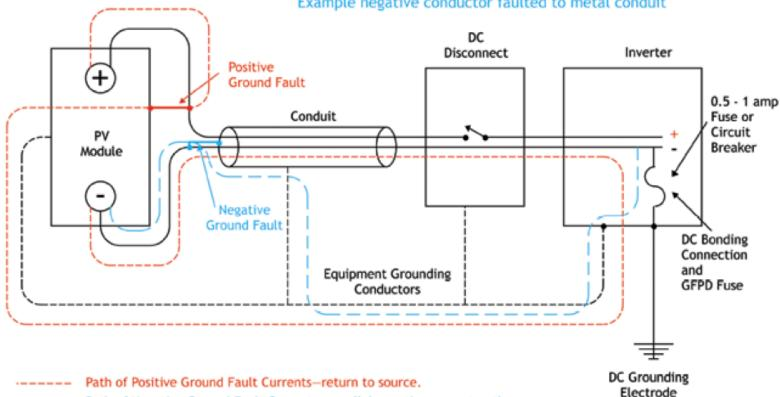
Path of Negative Ground Fault Currents-parallel negative current paths.
