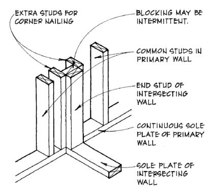
DOUBLE TOP PLATE OVERLAPS D CORNERS TO LOCK TWO WALLS TOGETHER. --2×4 STUDS 2 16 IH. O.C.
