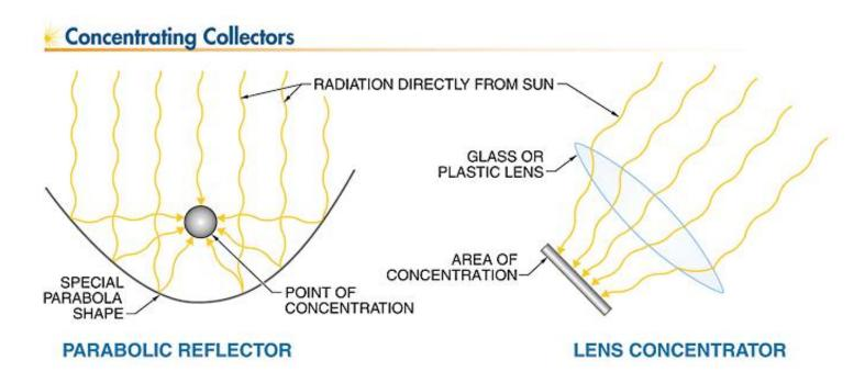
Concentrating collectors focus a large area of direct solar radiation onto a relatively small area.
