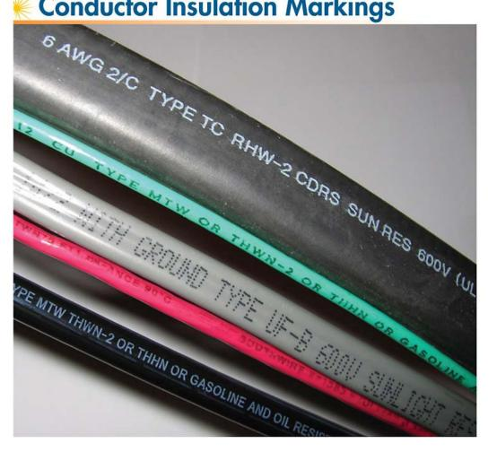
Conductor sizes typically used in PV systems range from 20 AWG to 2/0 AWG. Conductors may be solid or stranded.
